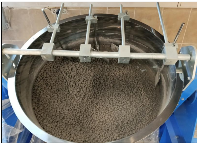
Figure 1. Disc pelletizer used to produce artificial aggregates.
