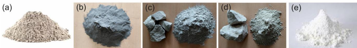
Visual 1. a. Clay, b. fly ash, c. acidic tuff, d. basic tuff, e. lime
