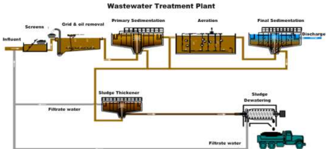
Figure 2. Wastewater treatment plant flow chart
