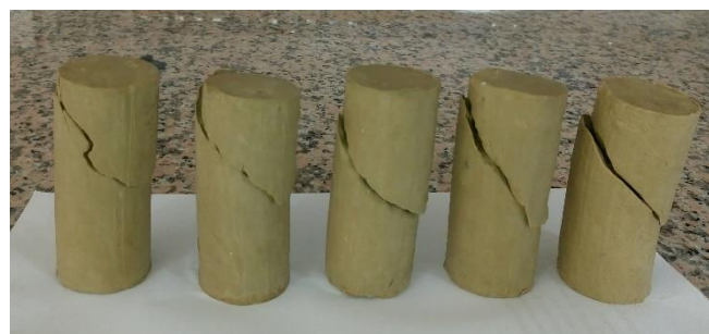
Visual 1. Failures determined in the samples after the triaxial compressive test
