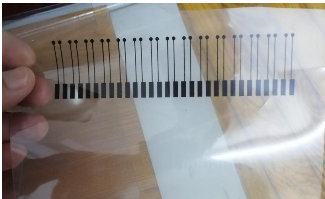
Figure 5. The final screen-printed model for potentiometric analysis in the lab
