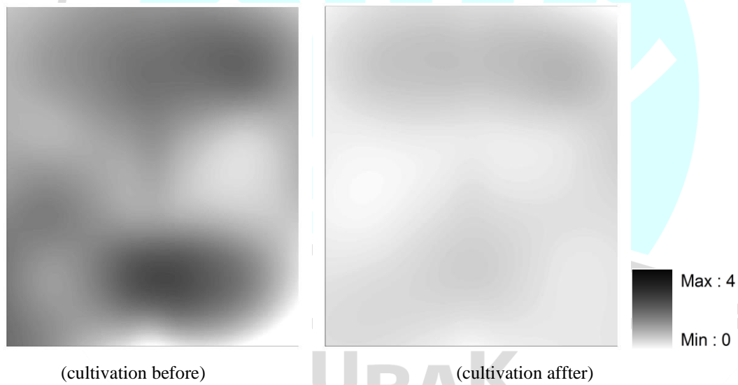
Figure 14. Penetration maps of standard subsoiler applications in vibrating mode (0-10 cm)
