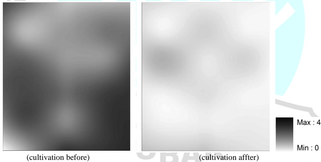
Figure 21. Penetration maps (10-20 cm) of subsoiler applications with knife chisel equipped in vibrating position
